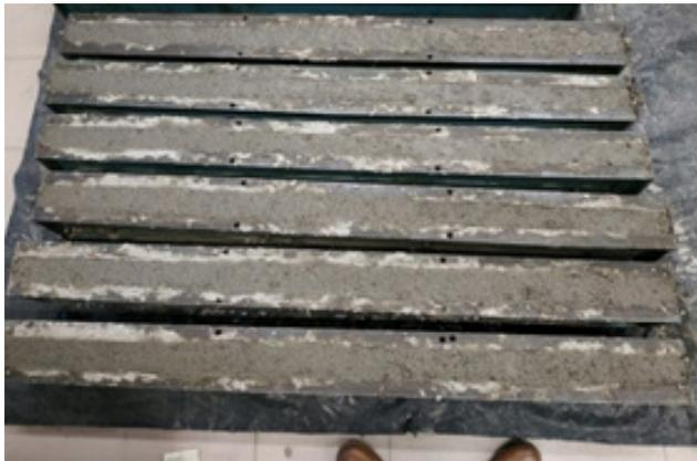
**Fig.1.** *Molding of Expanded Clay Concrete*
