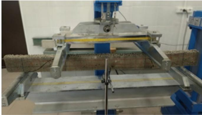
**Fig.3.** Deflection test on Expanded Clay Basalt Rod Reinforced Concrete Beam
