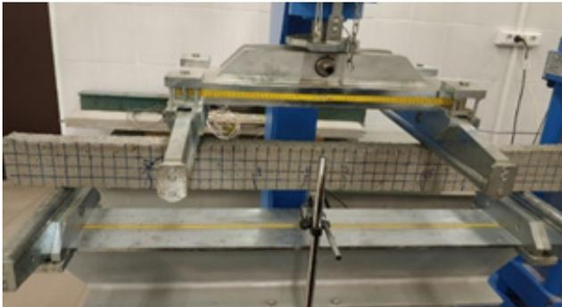
**Fig.5.** *Deflection test on dispersed Basalt Fiber expanded clay basalt rod reinforced concrete beam*
